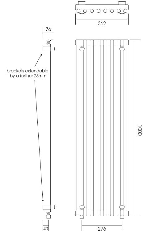
Width: 362 Depth: 76-99 Tube  $\varnothing$ : 35 + 23
